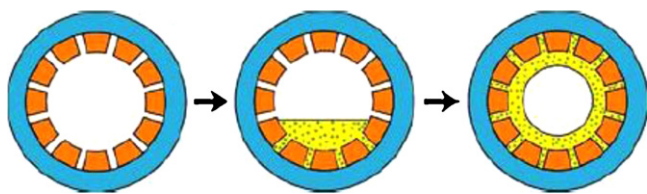
Fig. 6. Centrifugal casting of laser-perforated tubular SIS scaffold with in situ cross-linkable hyaluronan-based hydrogel and living cells.
